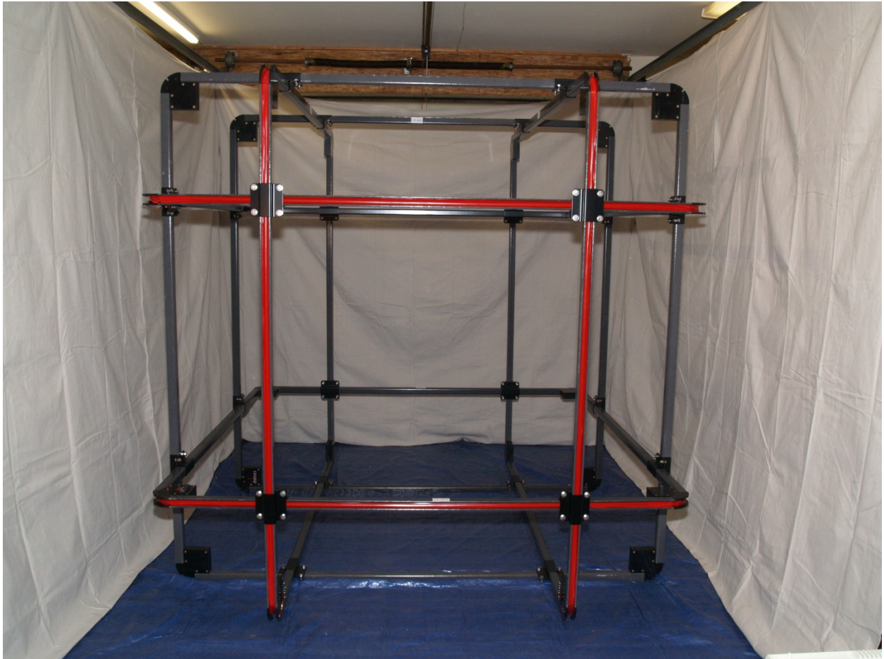
Coil Assembled with all the brackets attached.
