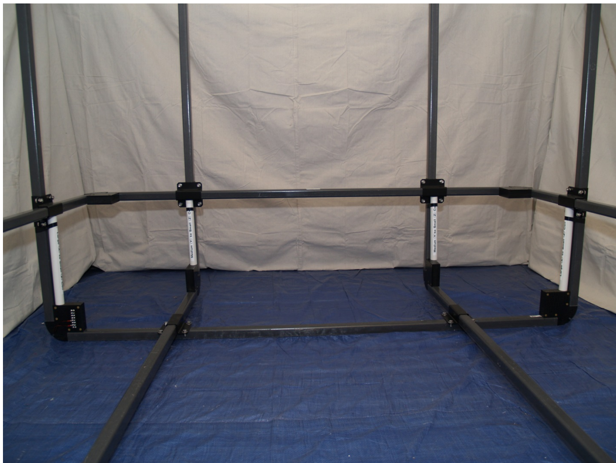
PVC tubes between +Z coil and X coils (opposite end)
