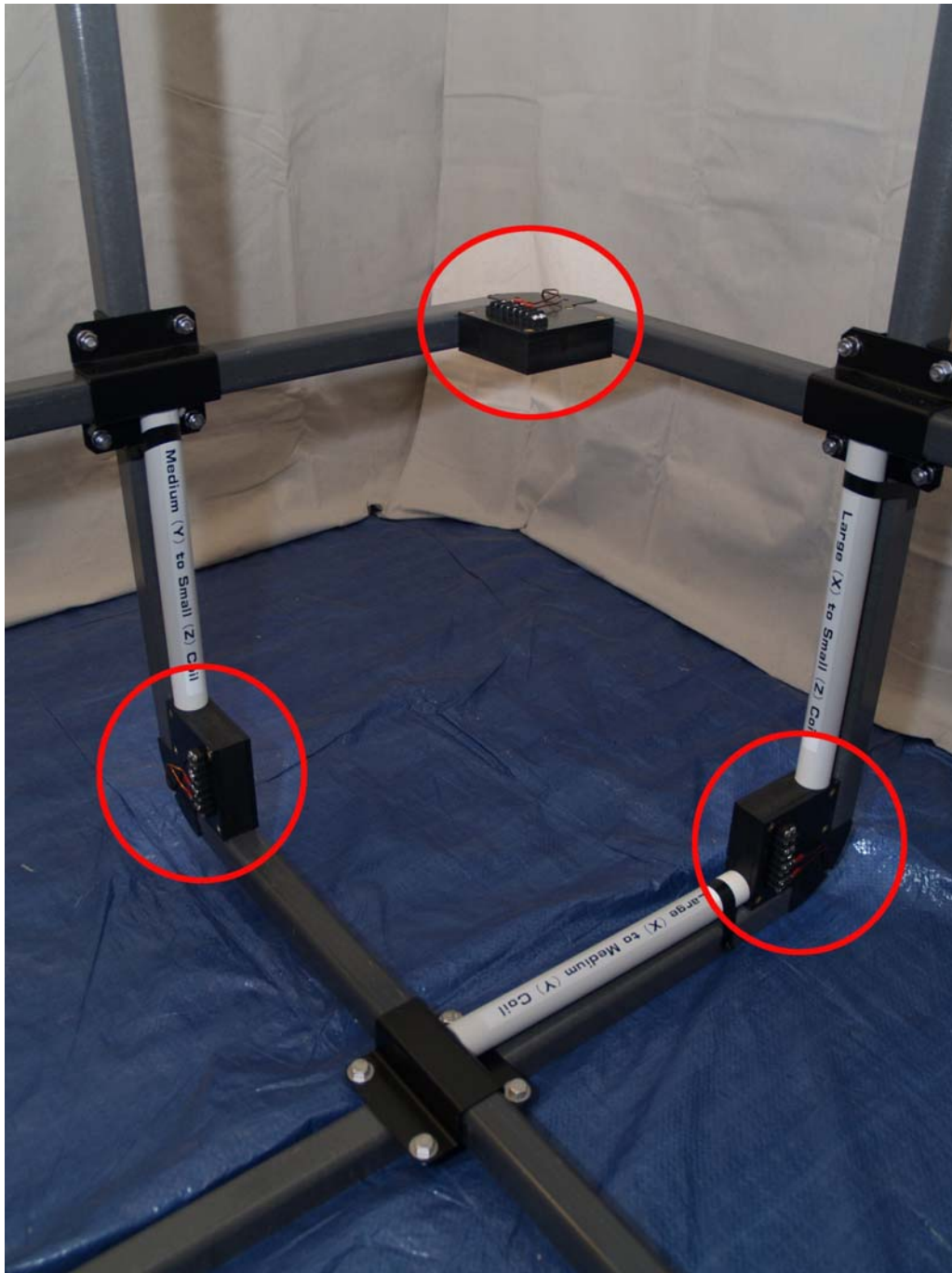
Coil corner -X , -Y , and +Z coil terminals
