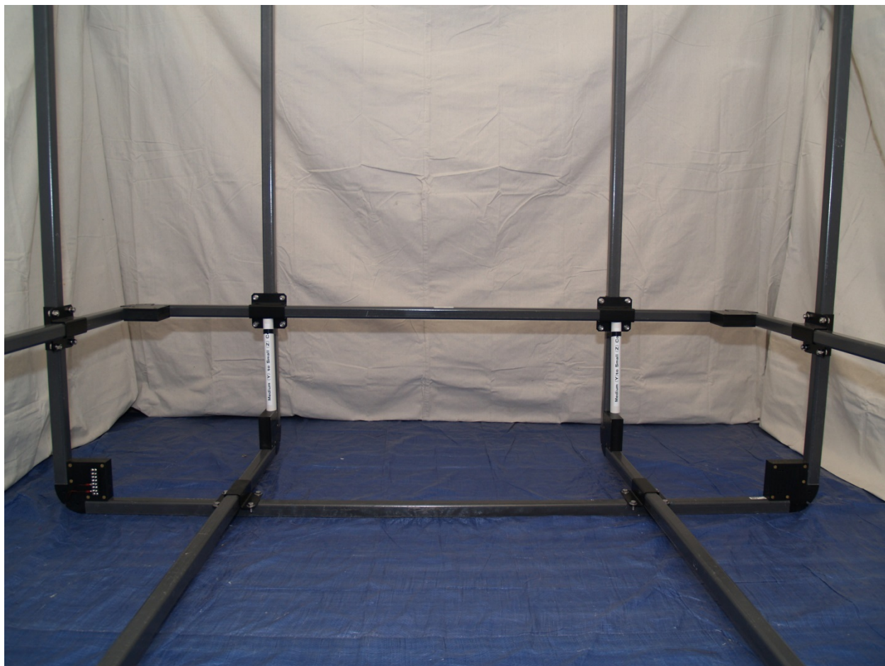
PVC tubes between +Z coil and Y coils (opposite end)
