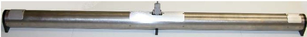
Figure 9 TRIGRAD Digital Gradiometer -1 Meter Baseline, Titanium Tube
